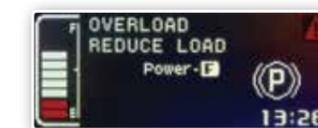
The weight value that appears on the load indicator should be read as a reference and not as the actual load weight.
